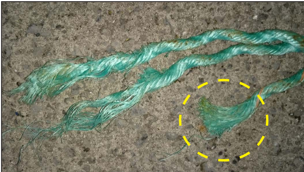
Figure 5: Broken back rope, indication that at least one strand had been cut
