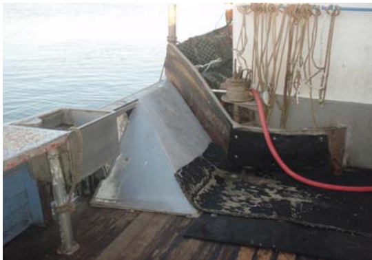
Figure 11: Self shooting ramp mid-ships onboard the Bridlington based vessel Nordstjerne
