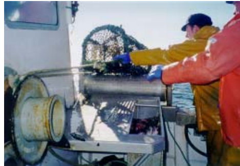
Figure 14: Hauling pots with roller
