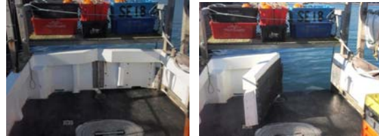
Figure 9: Shooting door open and closed
