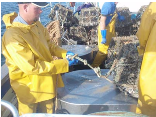
Figure 1: Detaching the pot from the main ground rope onboard 16m Dartmouth based vessel Excel
