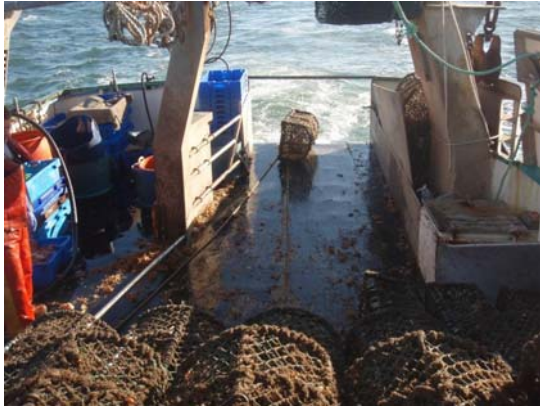
Figure 7: Self shooting through the stern opening
