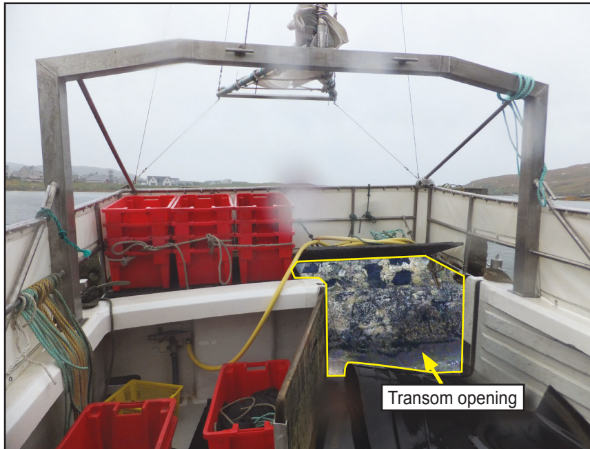
Figure 2: Transom, showing opening for shooting creels
