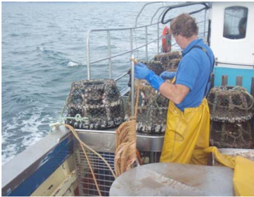
Figure 3: Attaching the pots to the ground rope whilst shooting.
