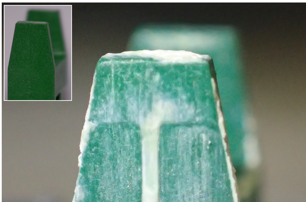
Figure 13: Close-up of moving part of switch from 'in' button on quarry side of wagon (inset shows corresponding view of new switch) (images courtesy of Schneider Electric)
