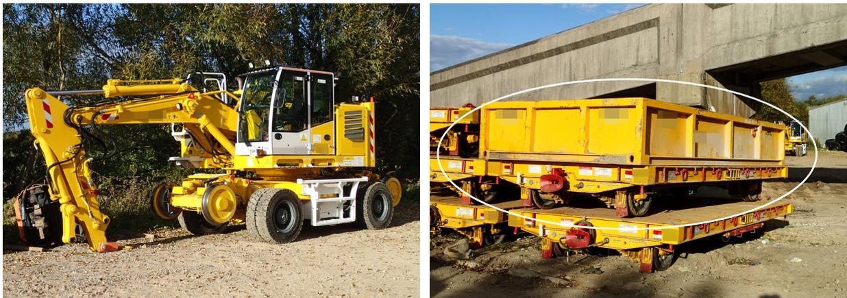
Figure 4: Example of a road/rail machine (left) and trailer and ballast box combination (circled right) similar to that used by the work group but not involved with the incident.
