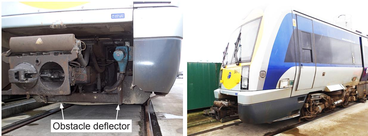
Figure 7: The front of train B301 after the accident
