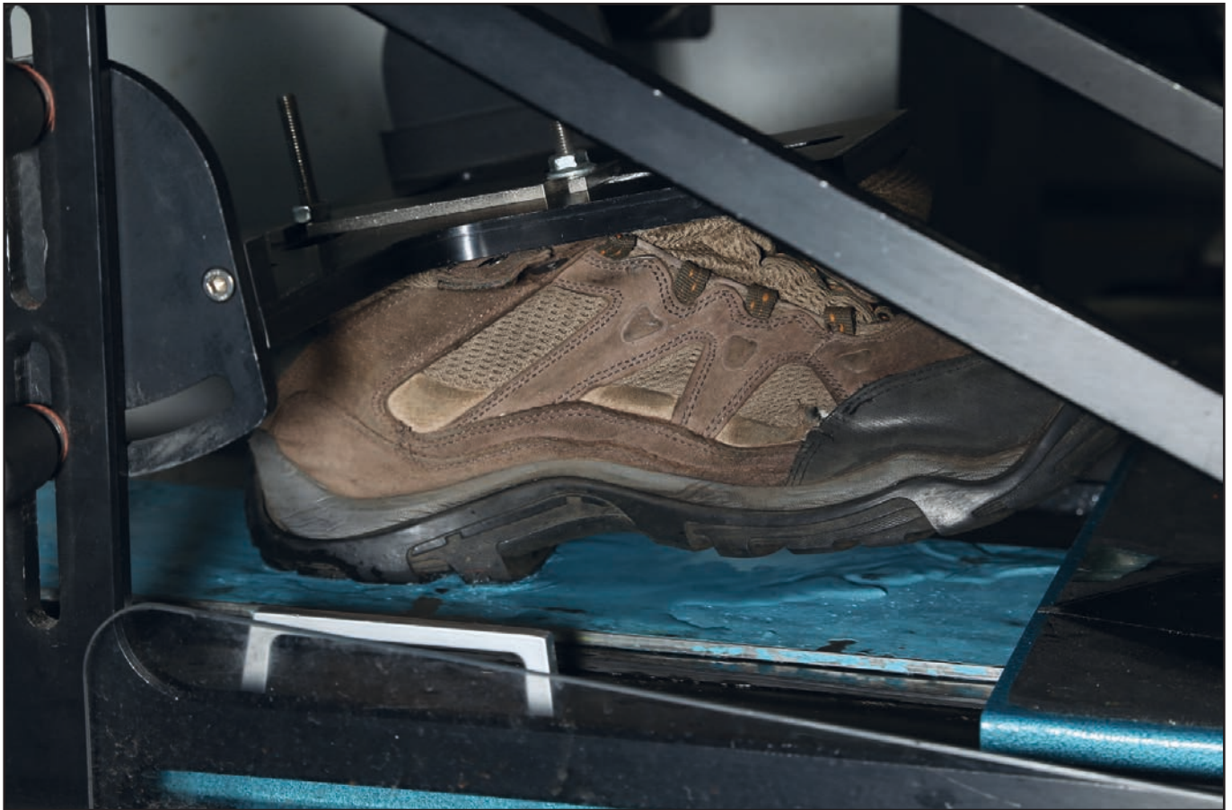
Figure 5: Walking boot undergoing slip resistance testing
