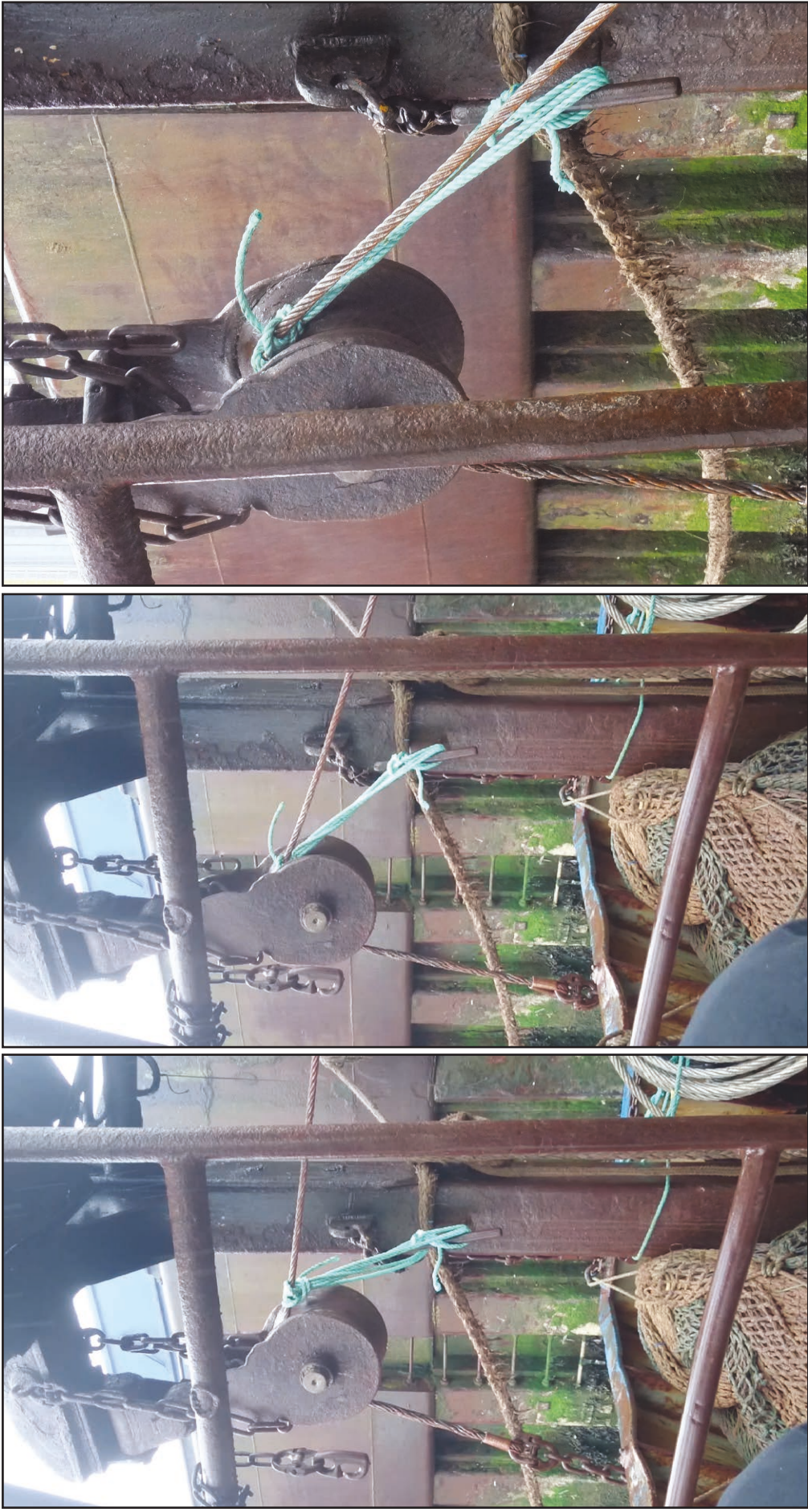
Figure 10: Reconstruction of stopper trapped in the gantry block as warp is veered
