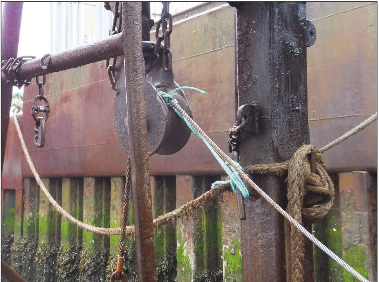
Figure 3b: Reconstruction of rope stopper trapped in block after warp slackened off
