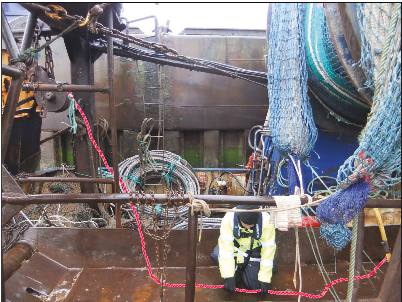
Figure 5: Reconstruction of marking the warp
