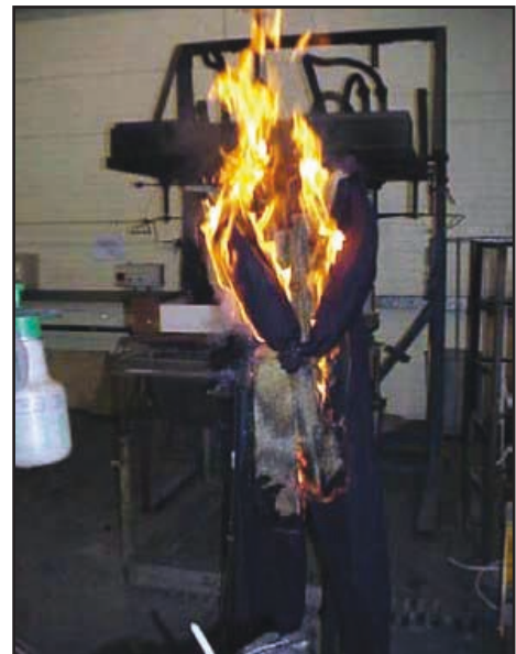
Figure 16: Coverall ignition and flame spread test after approximately 45 seconds (ignition occurred at approximately 20 seconds)
