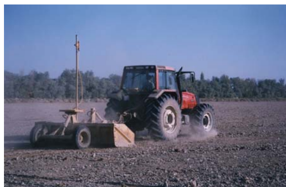
Machines for land levelling with laser
