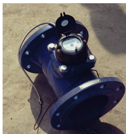
In-pipe water meter
