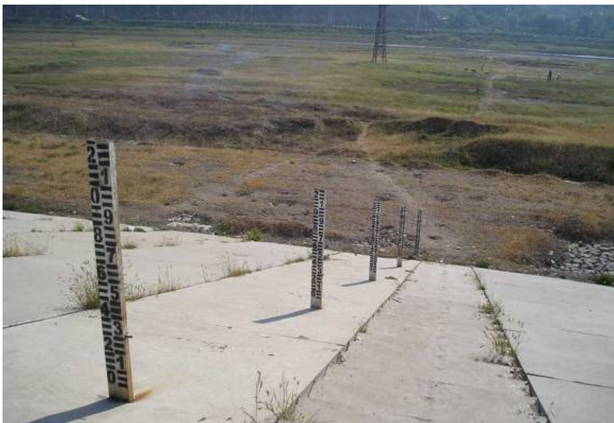
Gauging station in Liaoning
