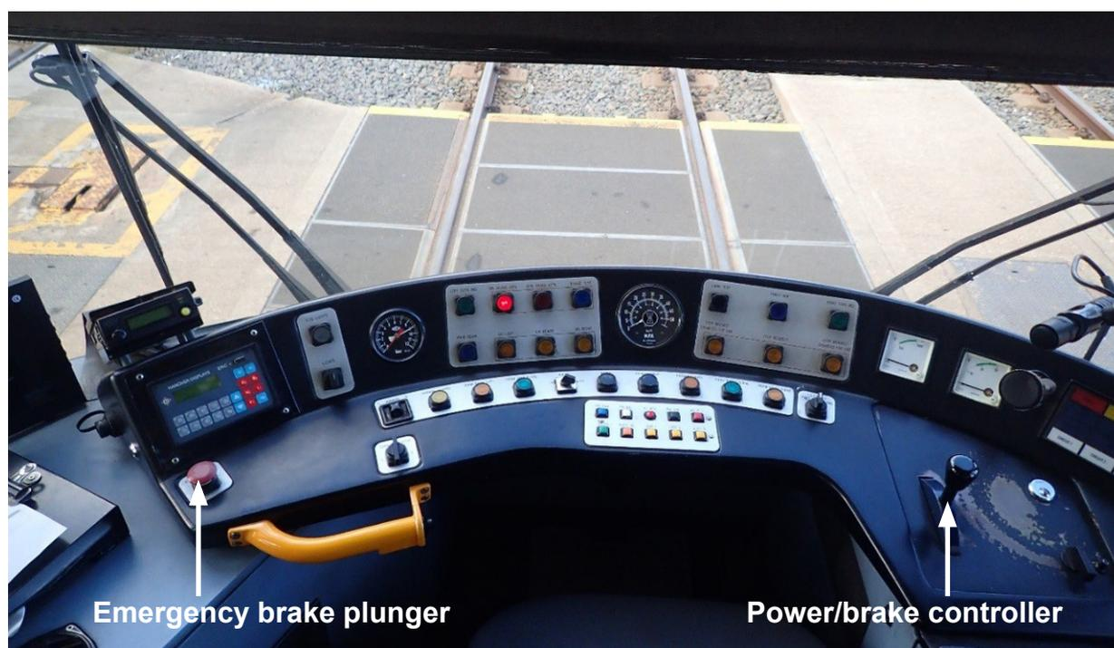
Figure 7: Layout of cab controls
