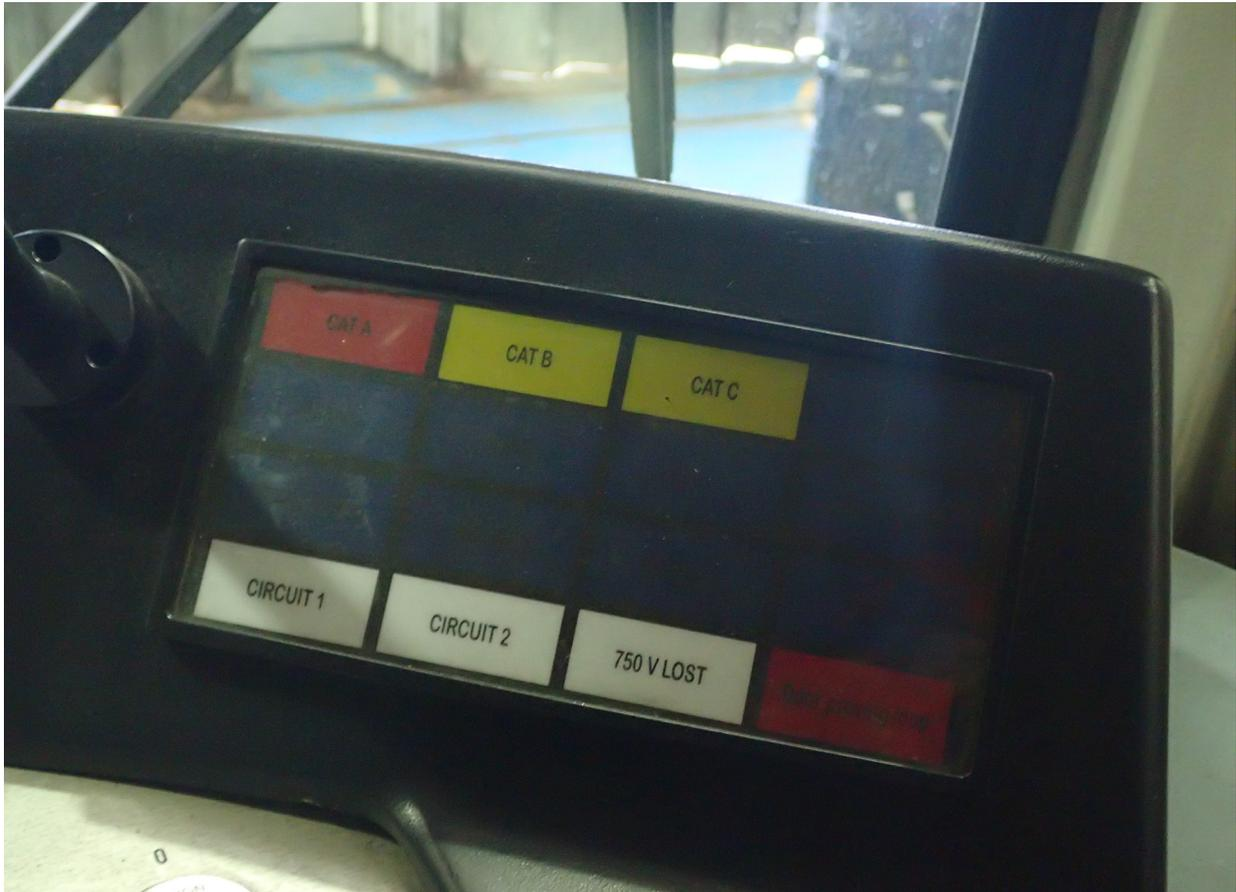
Figure 13: The cab annunciator panel
