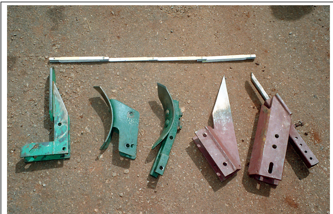
Fig 1 Designs of ripper tine (left to right: MR, BSPR, ZR, CKR, PS)
