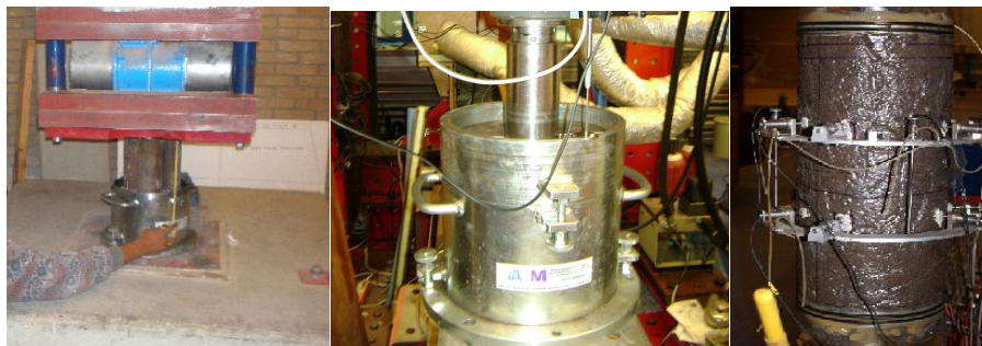
Figure 4: RL-CBR specimen during compaction (left), RL-CBR during testing (middle) and instrumented triaxial specimen ready for testing (right)
