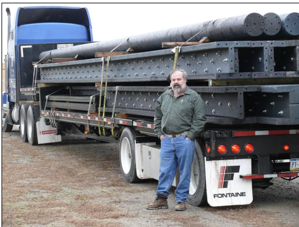
Figure 3: Plastic piers and I Beams prepared for transportation to site.
