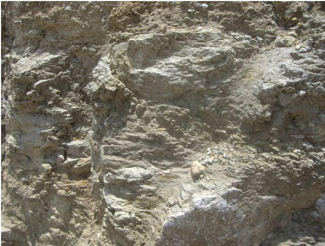
Figure 4 - Marly Limestone from BP 4
