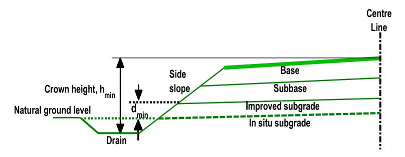
Minimum drainage requirements: hmin = +/- 750mm, dmin = +/- 100mm
