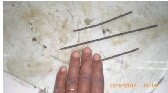
d. Rolling a soil thread for plastic limit
