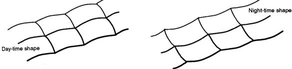
Fig. 13 Slab warping shapes
