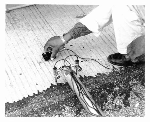
Plate 9b Close-up showing two vertical transducers and the gauge to measure horizontal strain
