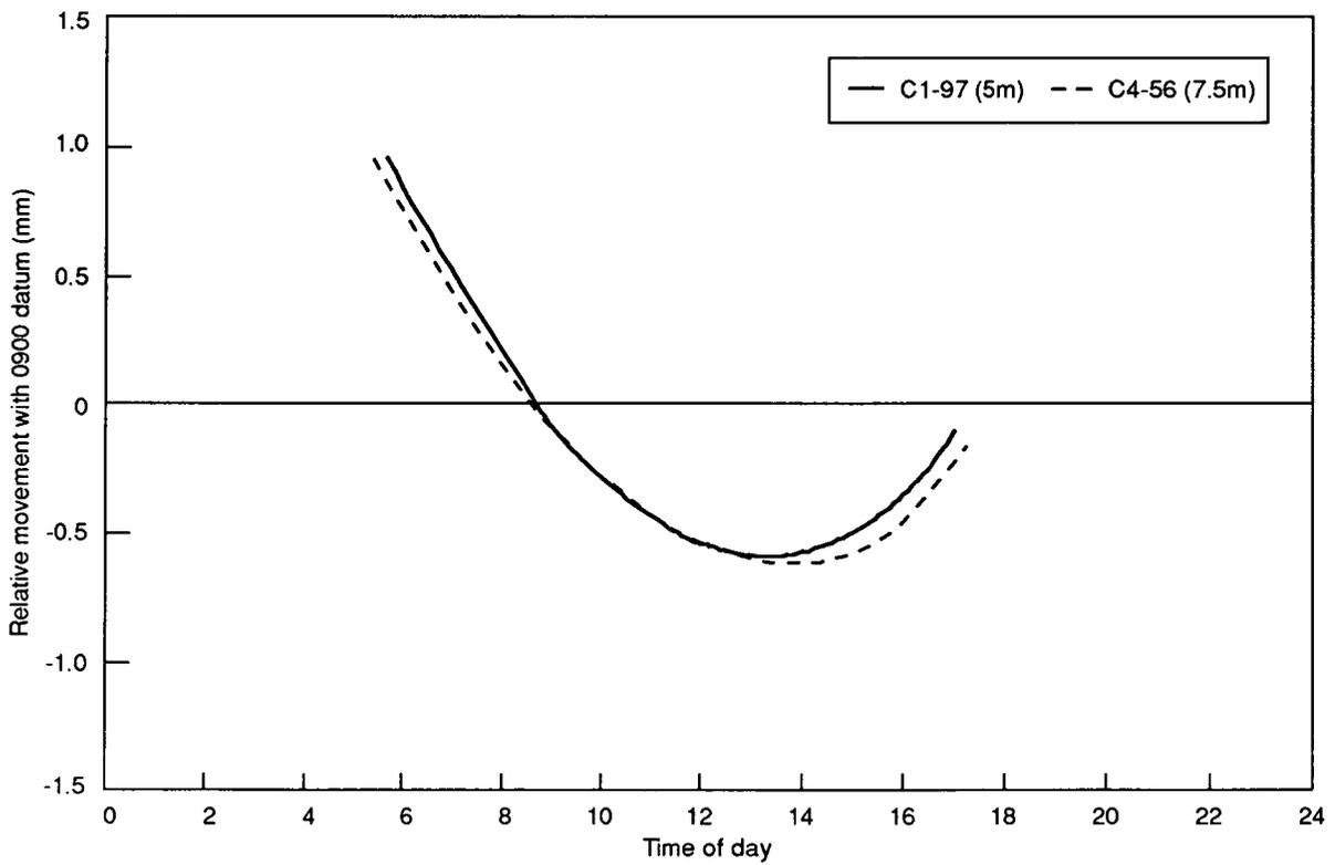
**Fig. 17 Longitudinal warping of slabs of different lengths**
