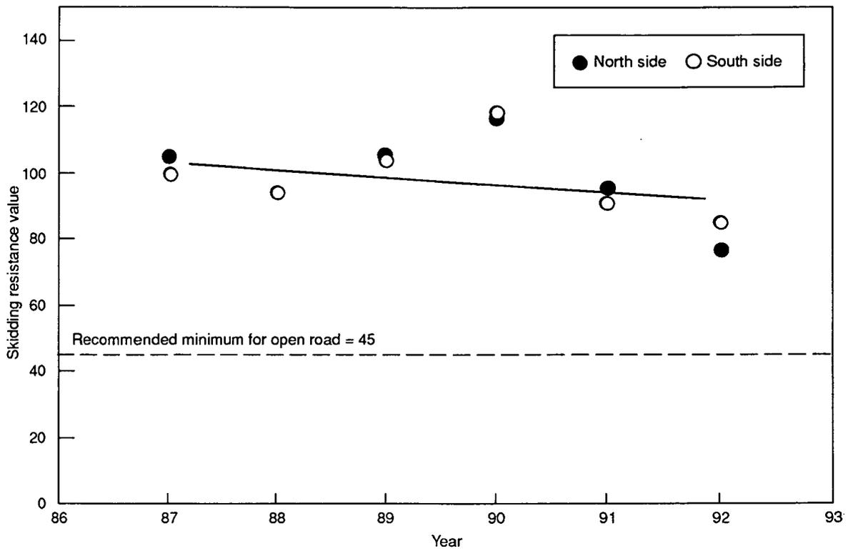
Fig. 4 Average skidding resistance (all sections)
