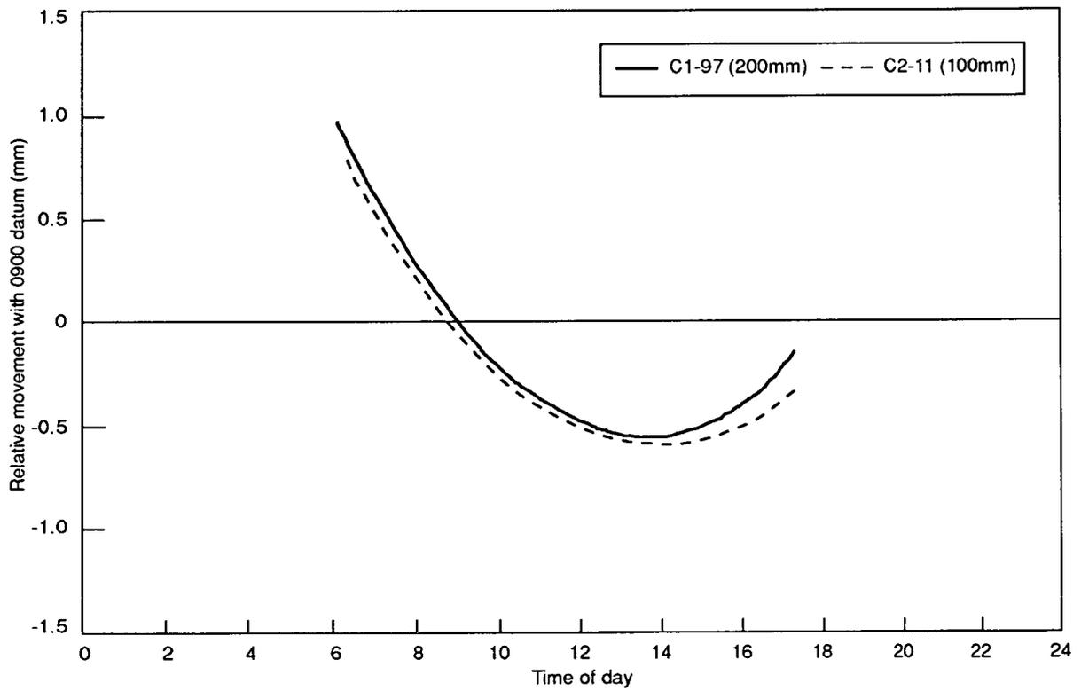
**Fig. 19 Longitudinal warping of slabs of different thickness**
