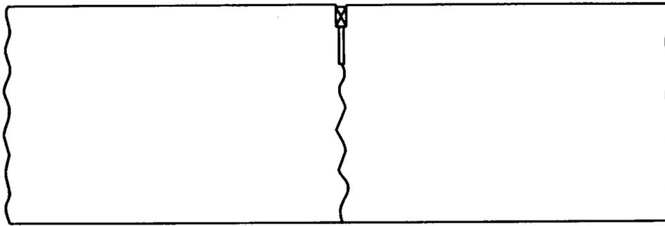
Contraction joints on Sections C1, C2, & C4 without dowels
