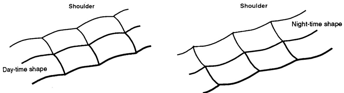
Fig. 13 Slab warping shapes
