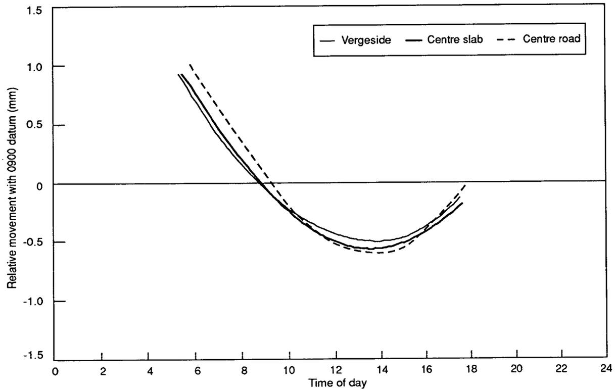
Fig. 15 Longitudinal warping of slab C1-97
