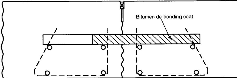
Contraction joints on Section C3 with dowels
