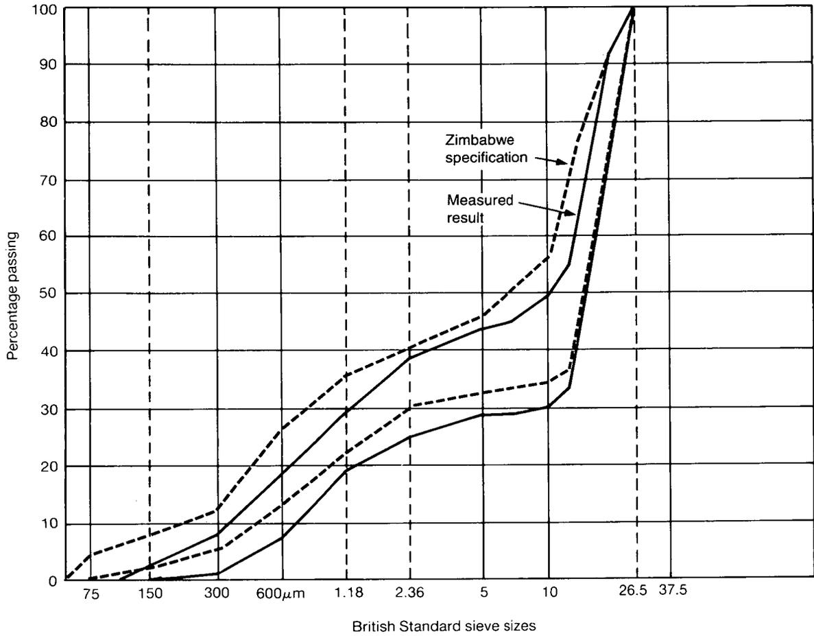
**Fig. A5 Wet sieving results – concrete aggregates**
