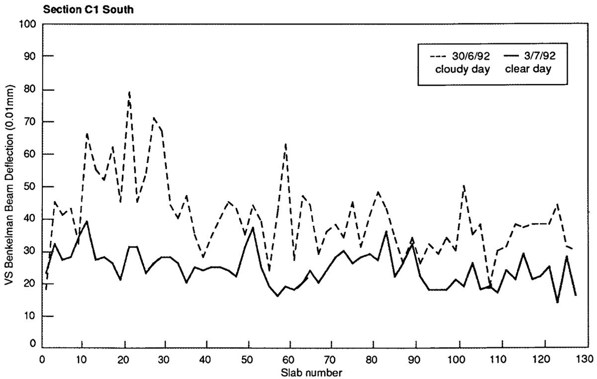
**Fig. 10 Repeat beam deflection measurements
