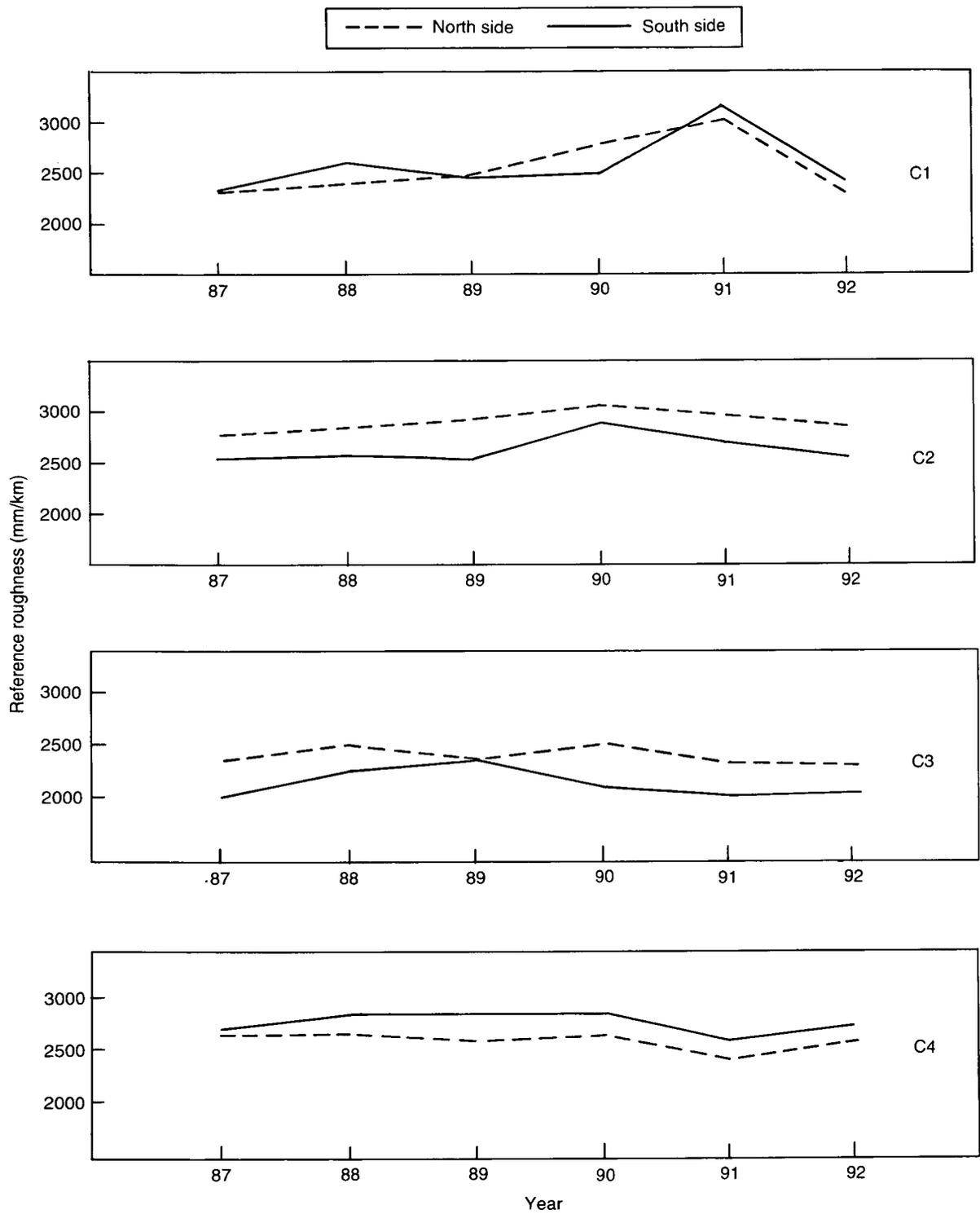
**Fig. 3 TRL profile beam roughness measurements**
