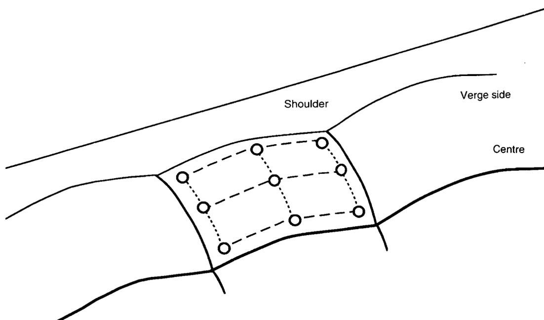
Fig. 11 Measuring points for slab warping
