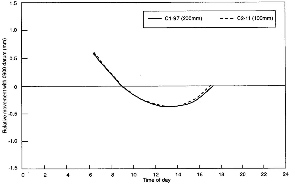
**Fig. 18 Transverse warping of slabs of different thickness**
