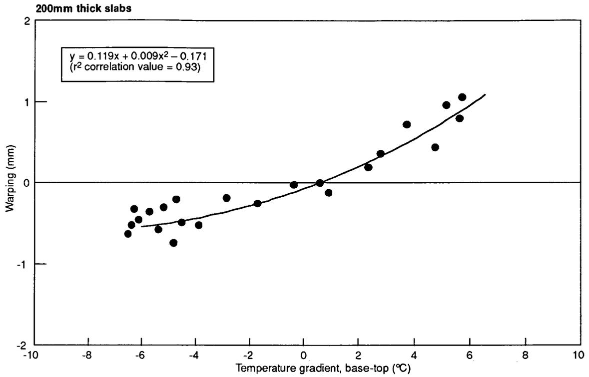
Fig. 20 Longitudinal warping plotted against temperature gradient (daytime)
