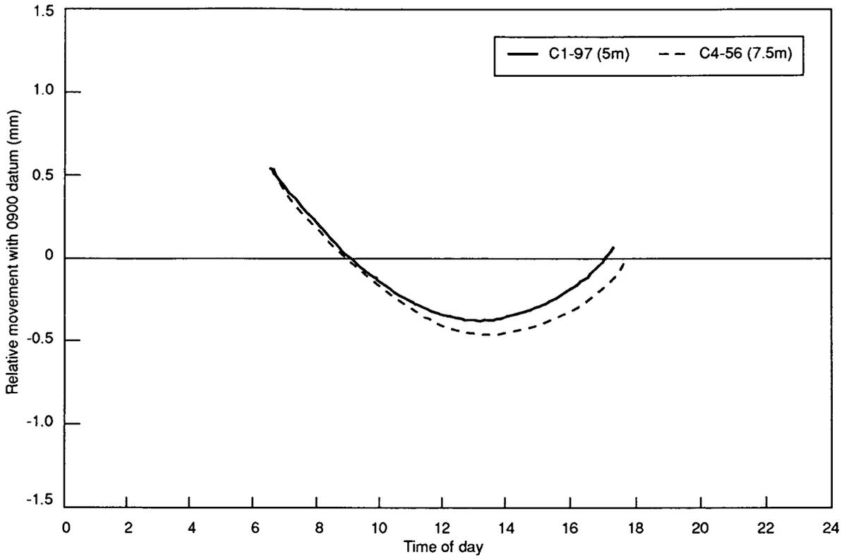
**Fig. 16 Transverse warping of slabs of different lengths**
