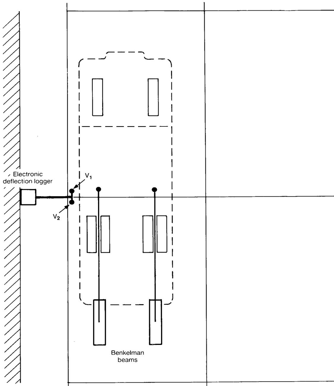
**Fig. 6 Instrument positions for deflection measurements**
