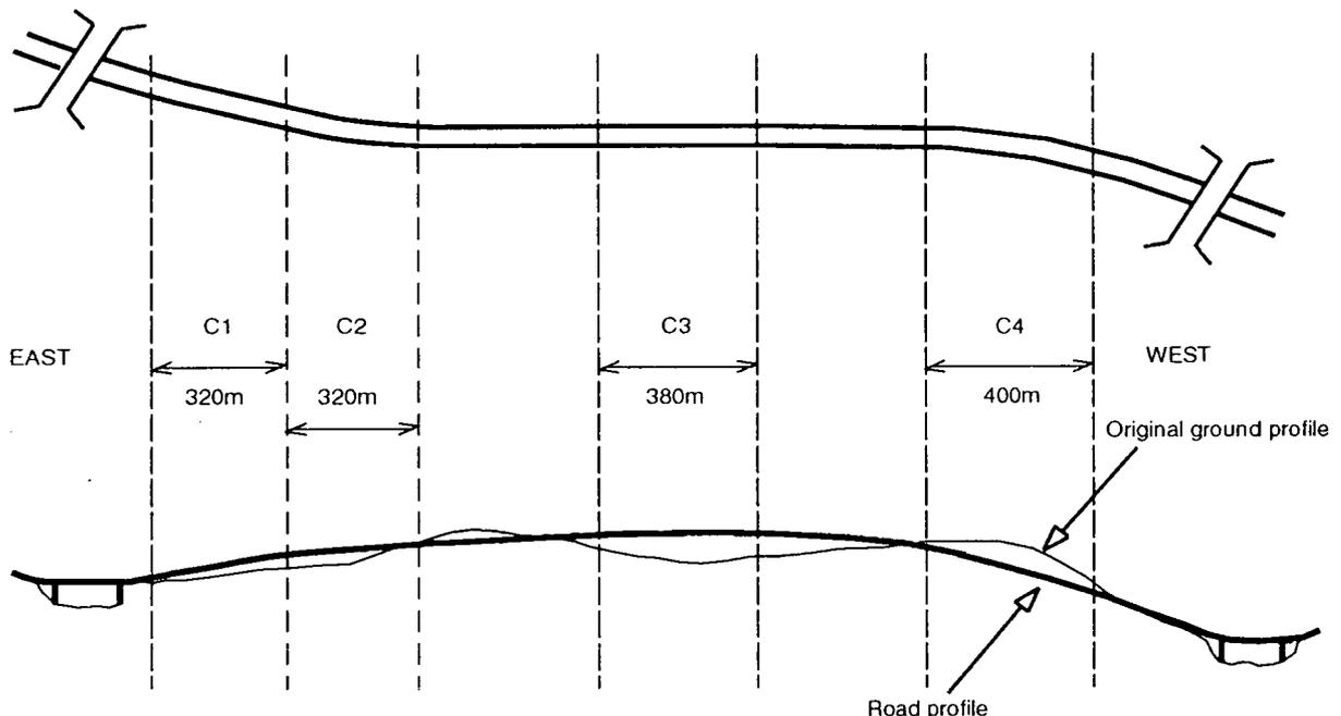
**Fig. 1 Horizontal and vertical alignment of the trial sections**
