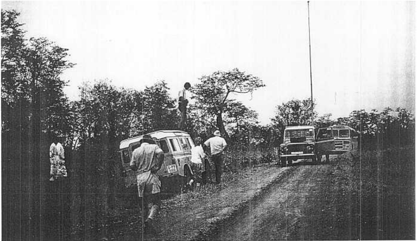
Plate 13. A marker party vehicle with telescopic mast partially erected.
