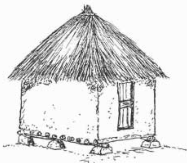
Figure 4. Examples of mud block/brick silos
