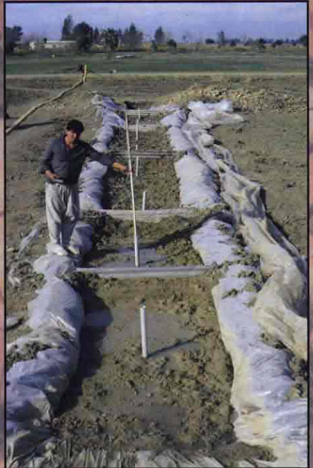
Trench trial, Seyhan, Turkey, showing position of bunds that encourage subsurface flow. Vertical pipesenable soilwater EC and the position of the saturation front to be monitored.
