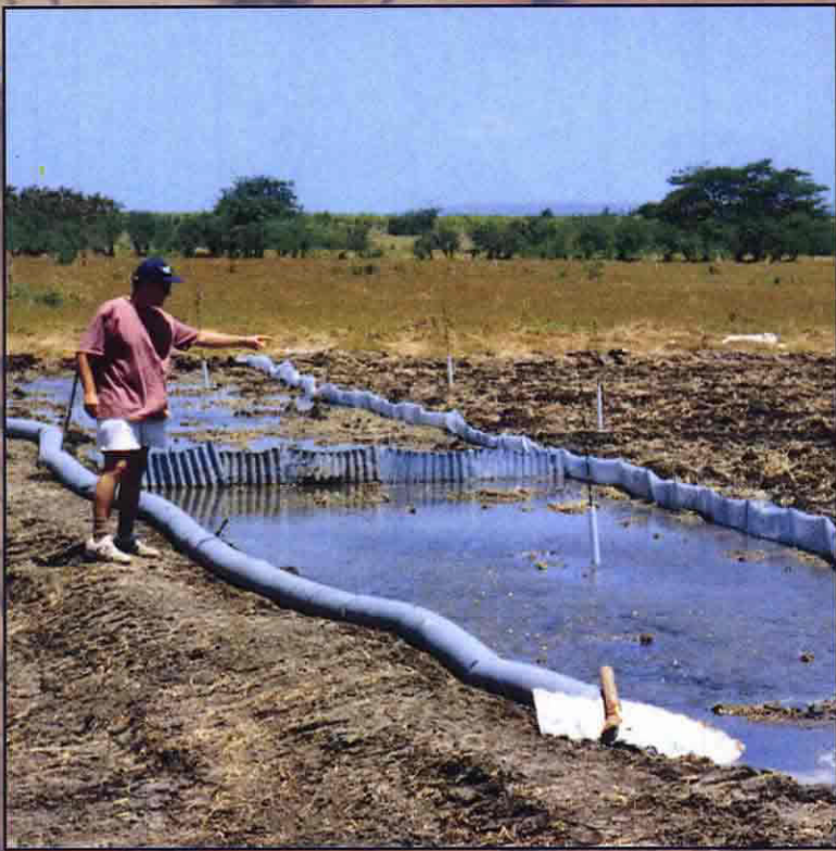
Plot trial, Jamaica, showing use of gated pipe (grey) to deliver water to the head pond. Vertical pipes contain float scales to indicate the position of the saturation front beneath the soil.
