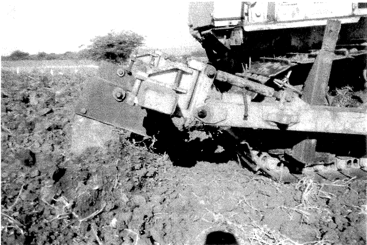
Plate 2 Tractor and subsoiler working at shallow depth
