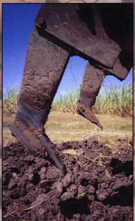
Double subsoiler used to shatter clay blocks into small aggregates.
