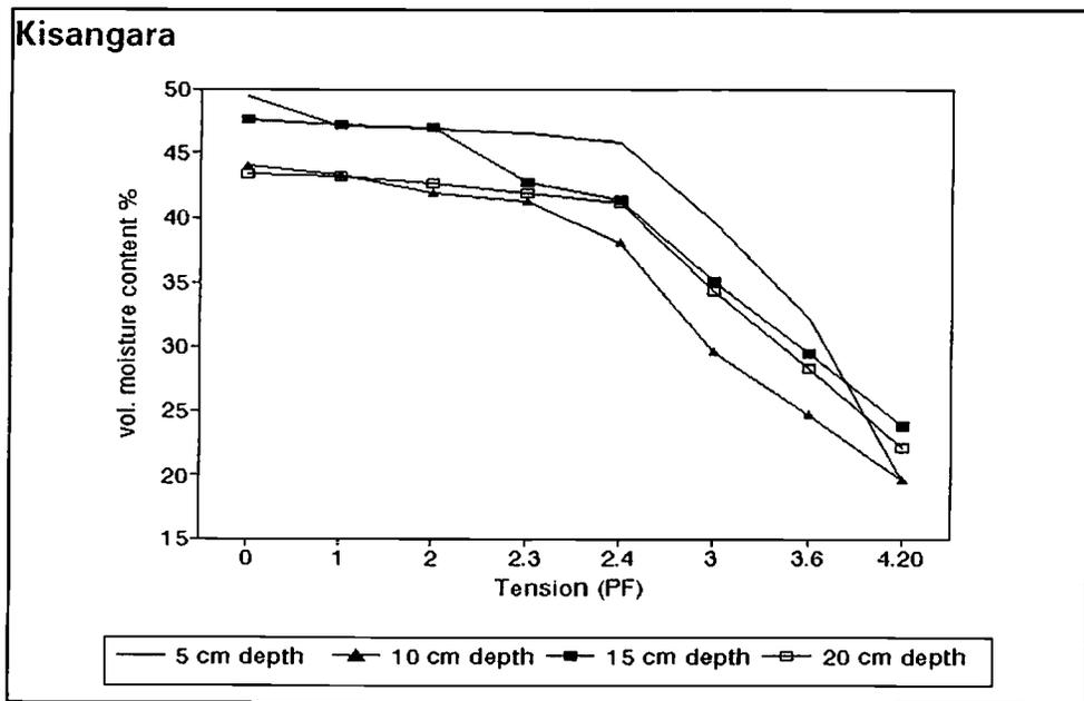
Figure 21. Effects of soil depth on Moisture release characteristics
