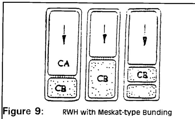
Figure 9: RWH with Meskat-type Bunding
