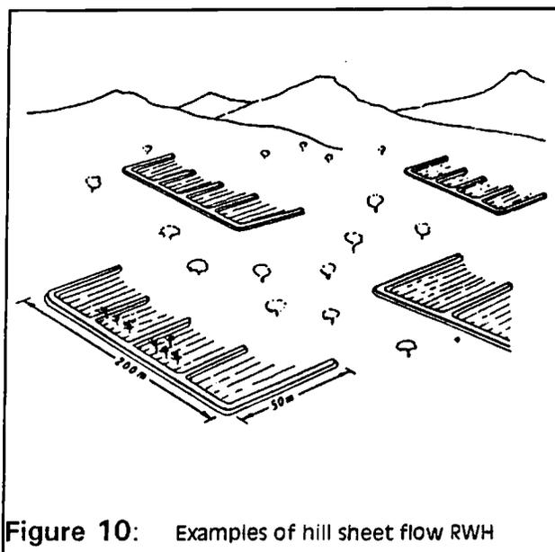
Figure 10: Examples of hill sheet flow RWH
