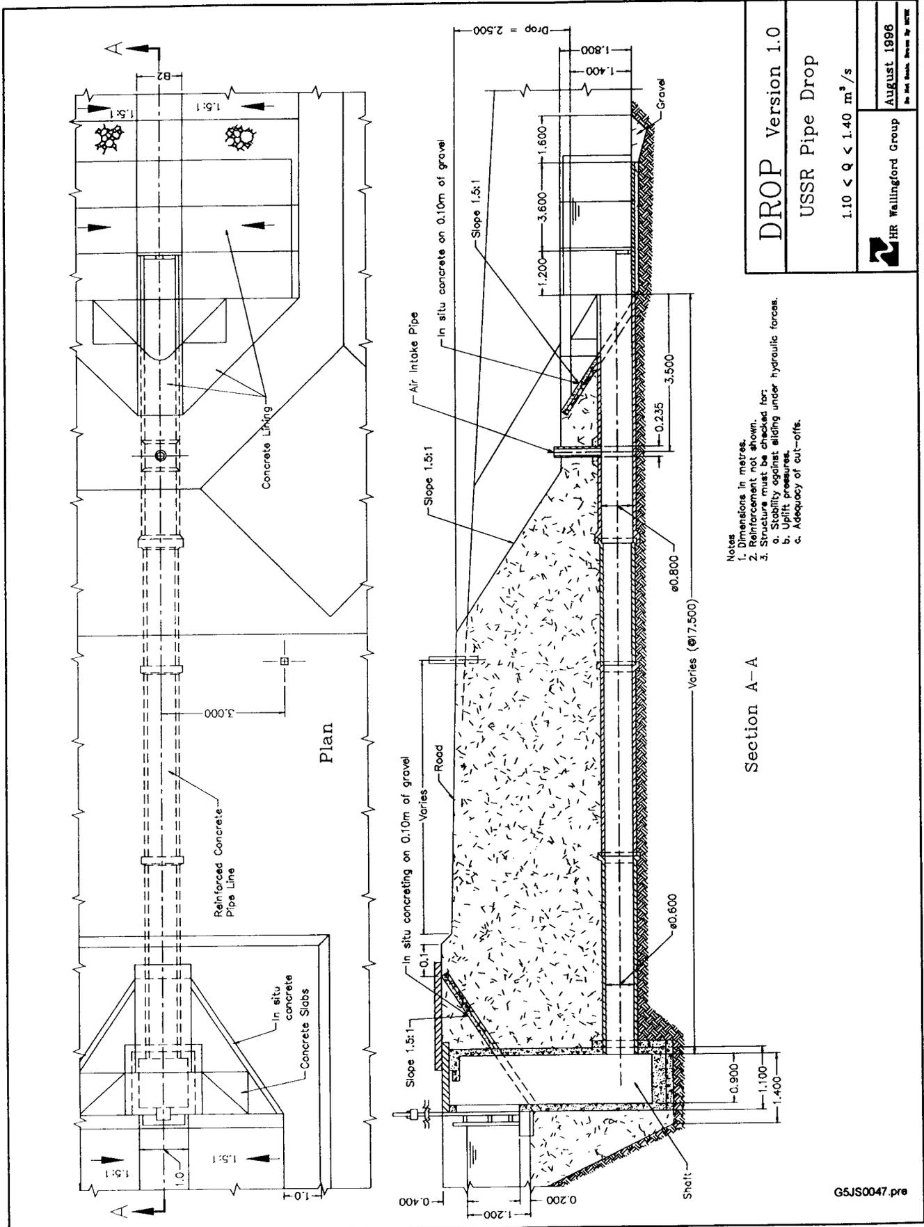
Figure 24 USSR Pipe Drop (after FAO)
