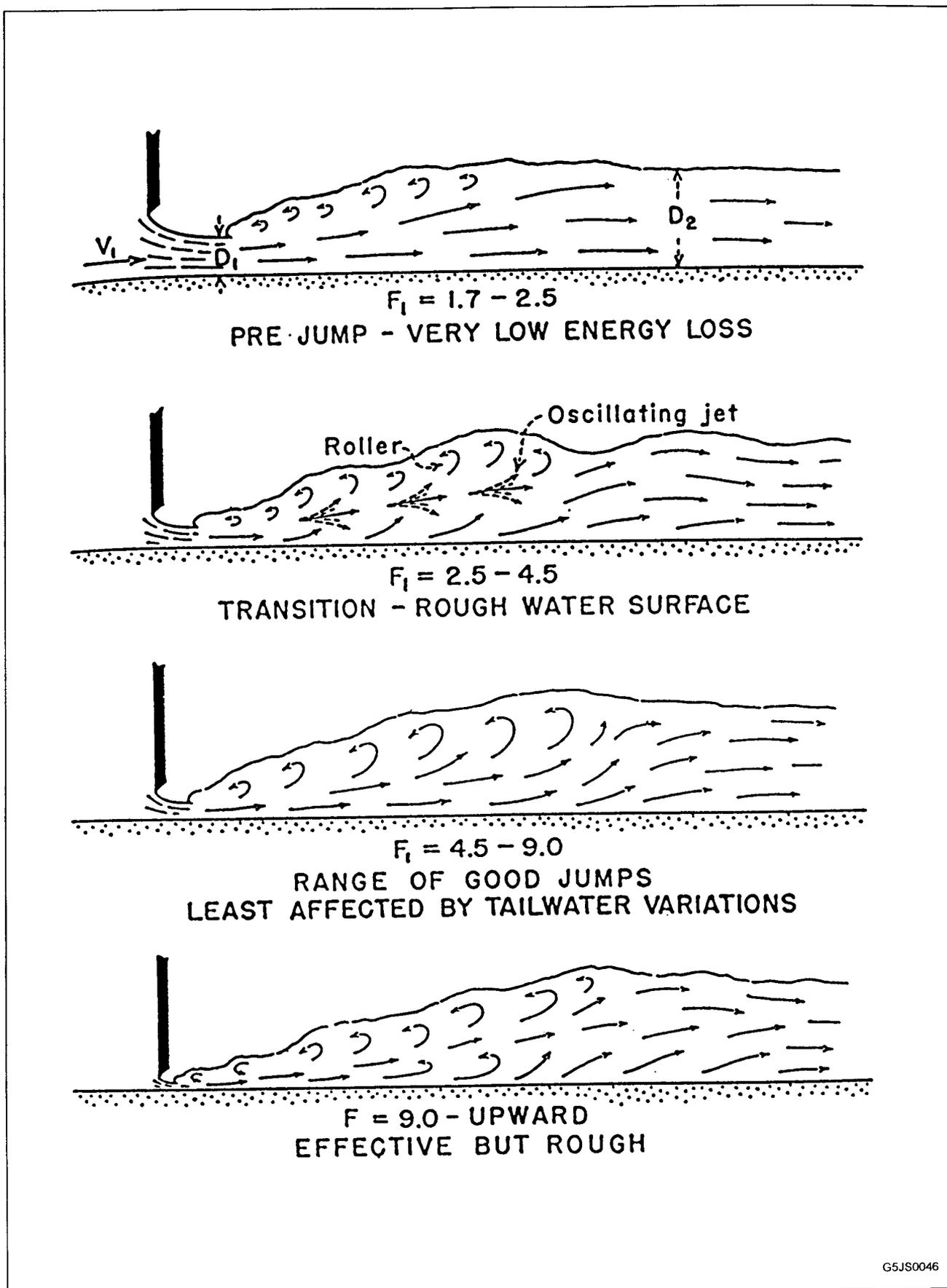
Figure 2 Varying forms of the hydraulic jump with increasing Froude Number (after USBR)
