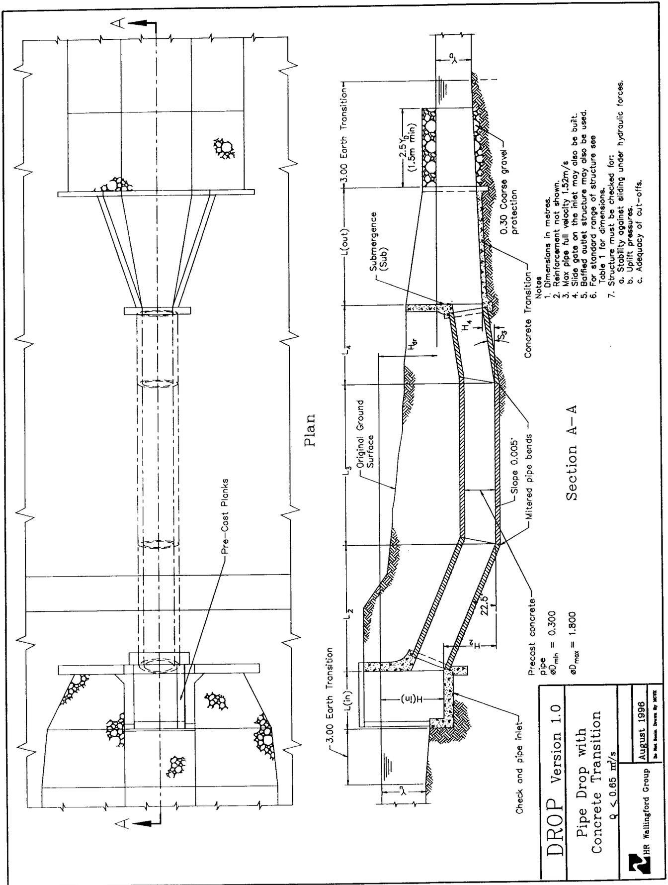
Figure 25 USBR Pipe Drop with Concrete Transition
