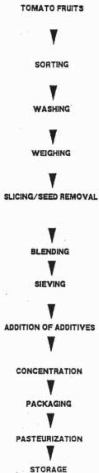
FLOW DIAGRAM FOR PASTE PRODUCTION (PROCESS A)
