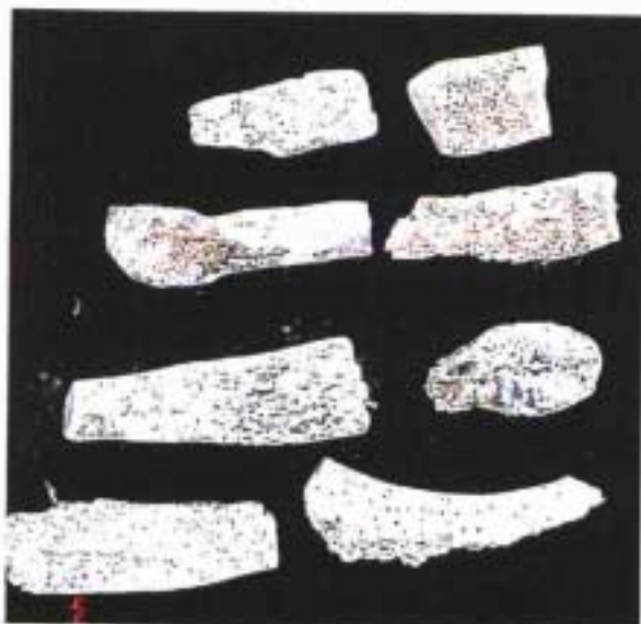
(c) Class 4 - medium-high damage
