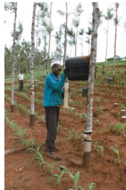
Plate 3.7: Measuring the amount of rainfall that was channelled down to the soil along the trunk (stemflow).
