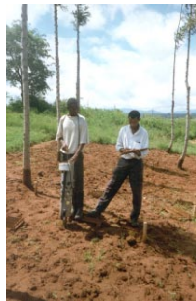
Plate 3.15: Measuring the volumetric water content of the soil profile using the neutron probe. Measurements were carried out weekly by ICRAF personnel.
