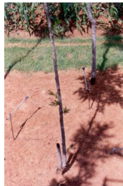
Plate 3.7: Measuring the amount of rainfall that was channelled down to the soil along the trunk (stemflow).
