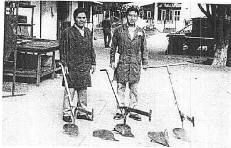
Fig. 14: Prototype production complete — Edgar Cafari and Porfirio Gamez with green plough: CIFEMA frame and 6" body, 4 ½" body (fitted), riding body: blue plough
