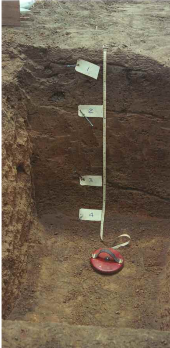
Plate 6.1 Trial pit dug through dense borrow area showing soil profile
