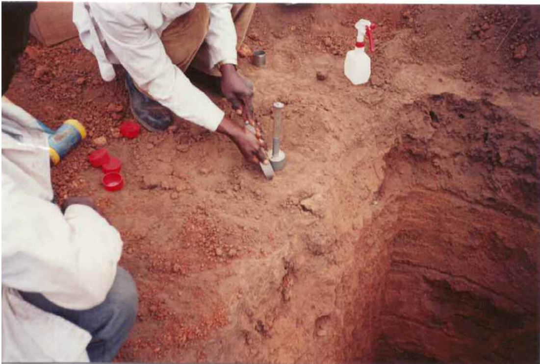
Plate 6-5 Extraction of undisturbed soil cores for in situ soil density testing
