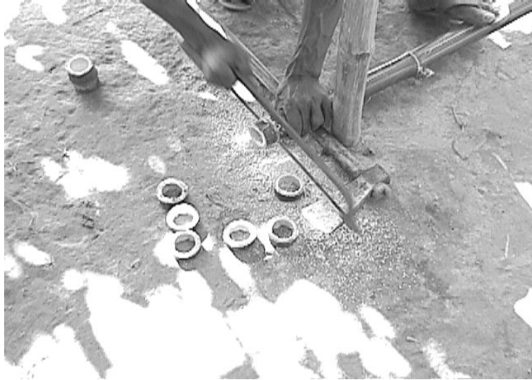
Figure 12: Cutting the Bamboo “Doughnuts”
