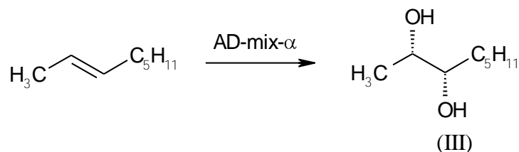
SCHEME 2. Synthesis of (S,S) -2,3-dihydroxyoctane (III)
