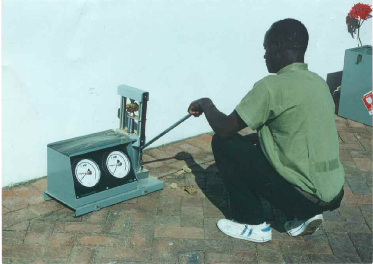
Plate 4-3 Point load testing of stabilised roadbase
