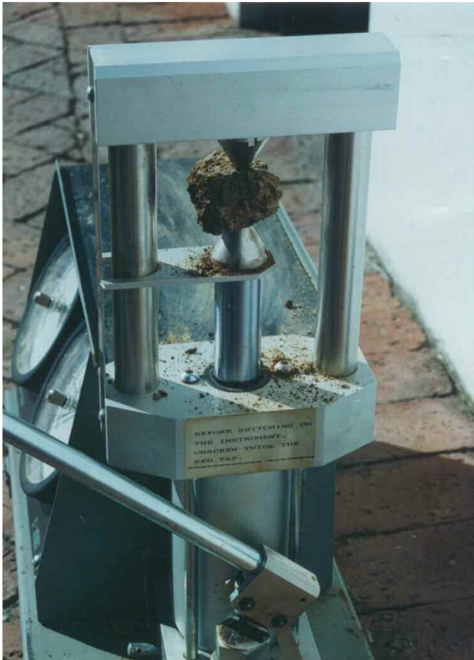
Plate 4-4 Point load testing of stabilised roadbase
