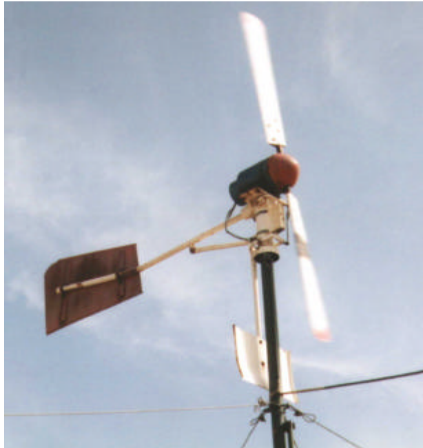
Figure 16 A lady bought a second hand replacement blade that had been welded (lower blade).
