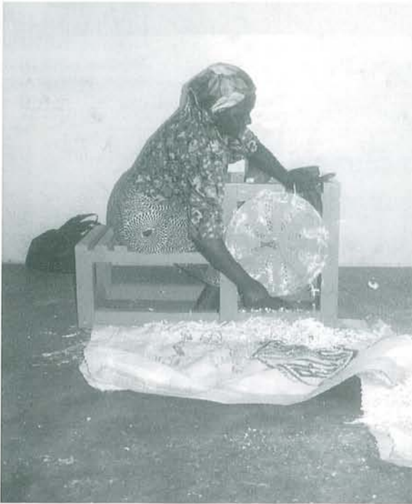
Fig. 1. Wooden framed cassava mini-chipper.
