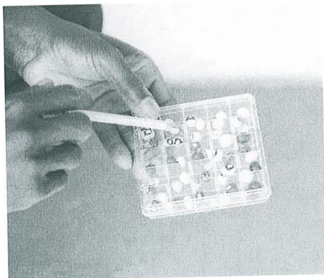
Figure 5. Titre block used for examination of pulse samples
