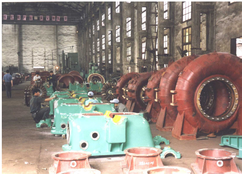
Standardised Francis and Pelton casings at the Jinhua Hydraulic Machinery Factory
