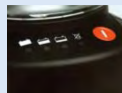
Four LED indicators displays status (battery full, battery good, battery low, lamp off)
