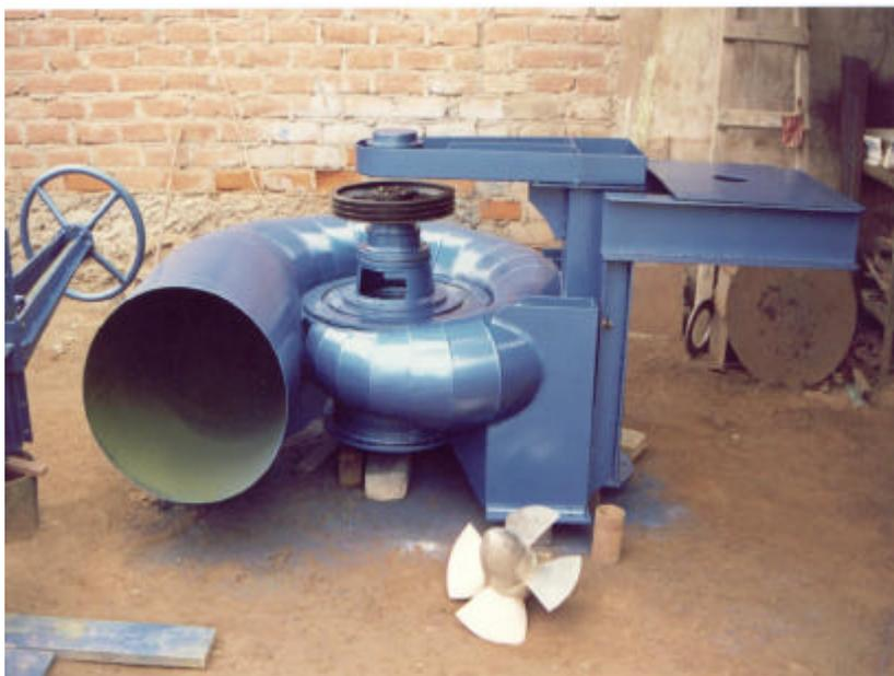
Figura 14: Turbina axial terminada
