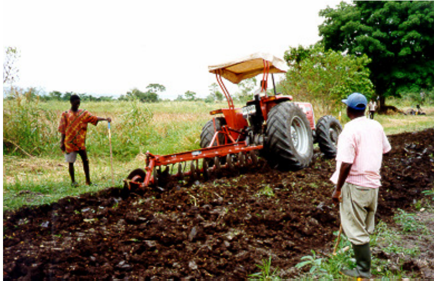
Plate 2. Tilling a camber bed with a polydisc
