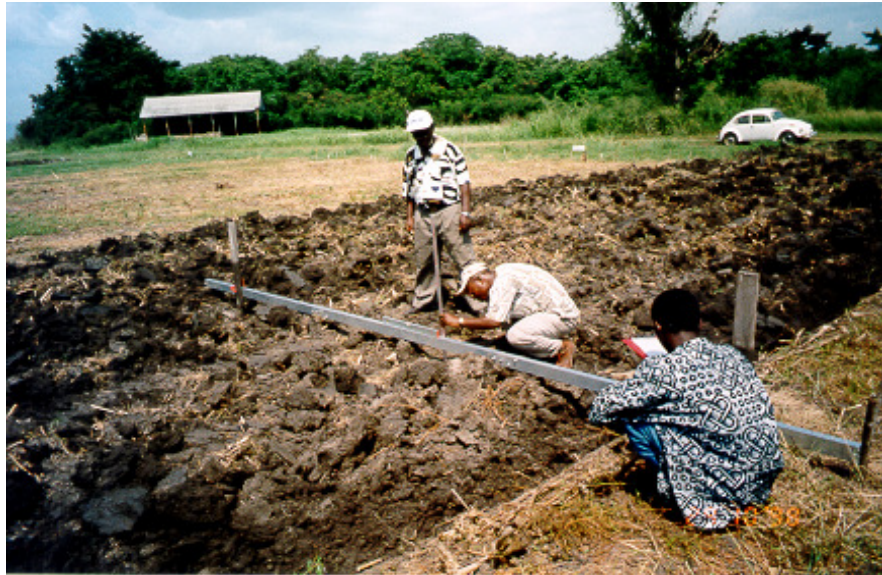
Plate 4. Measuring a soil surface profile with an aluminium beam
