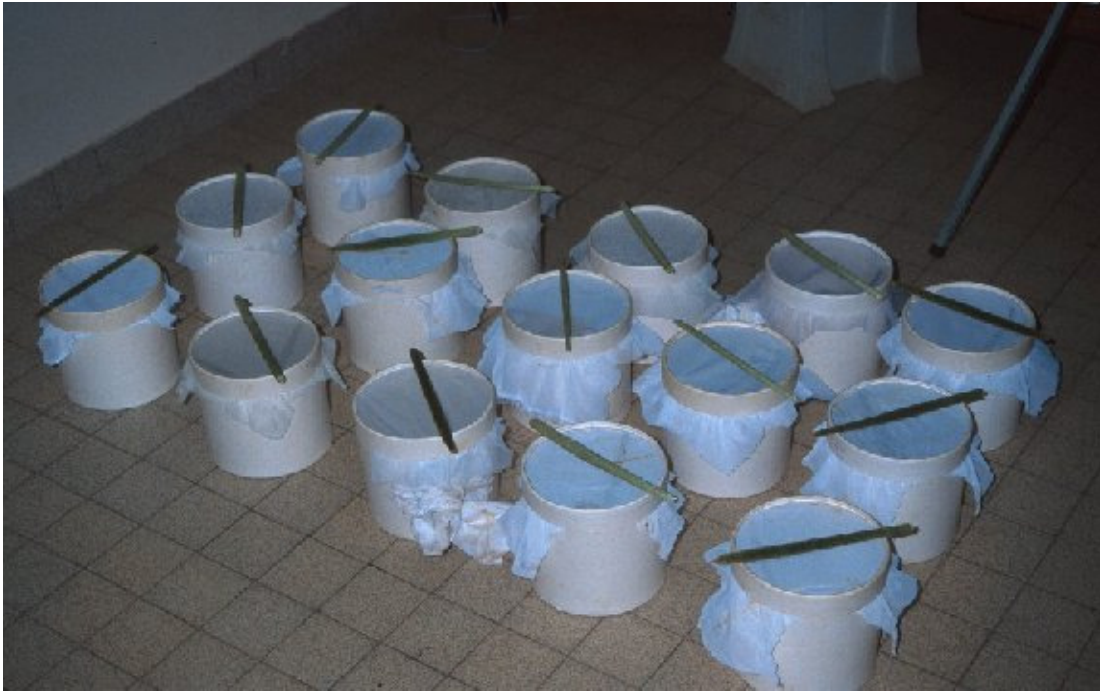
Figure 2. "Small cages", each containing two methanol-extracted panicles and a female H. albipunctella . The fresh panicle positioned on top of each lid provides a source of volatile chemicals - the smell of fresh panicle. The control treatment (no fresh panicle) was set up in a different room.
