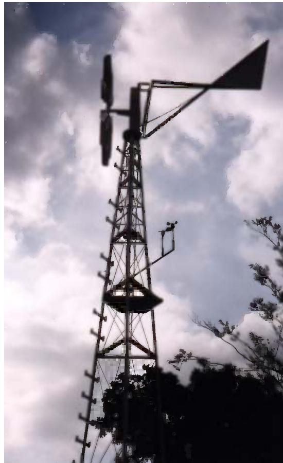
Figure 3.3: The IT Power windpump in South Africa with the anemometer and windvane
