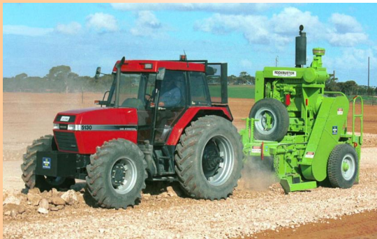
Rockbuster mobile hammermill treating oversize on the road (Photos Courtesy of Broons Hire (SA) Pty Ltd)
