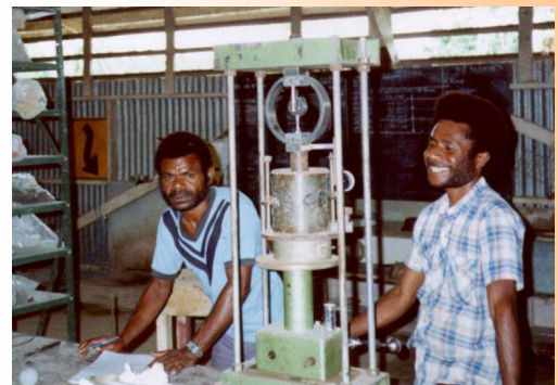
CBR test in progress, using a simple manually operated apparatus.
