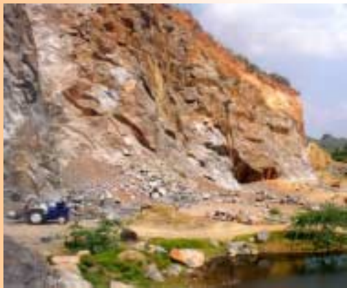
Example of poor quarry practice. Benched rock quarrying makes excavation easier and safer and limits scarring of the landscape by allowing more effective reinstatement.
