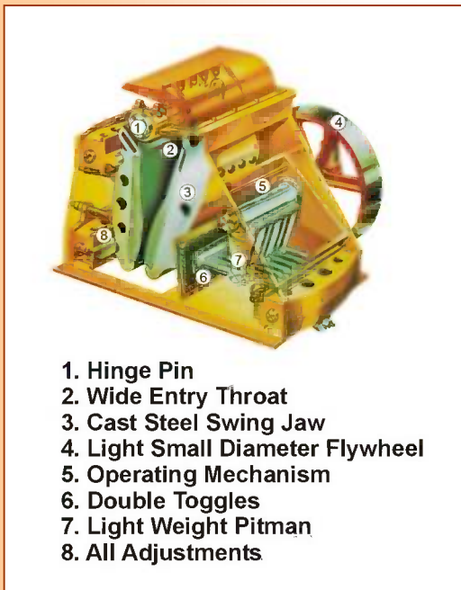
Section through a Double Toggle Jaw Crusher (Source: BL Pegson)
