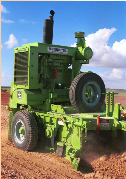
Rockbuster mobile hammermill treating oversize on the road (Photos Courtesy of Broons Hire (SA) Pty Ltd)
