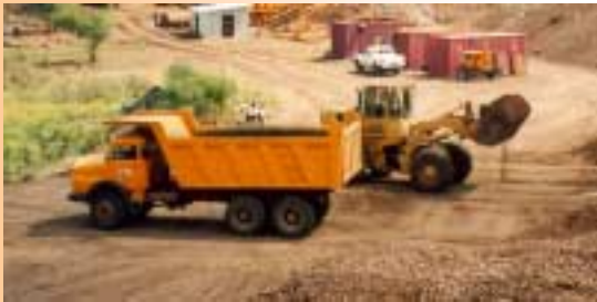
Wheeled front end loaders are ideal for excavating and handling loose soils and gravels in borrow and stockpile areas.
