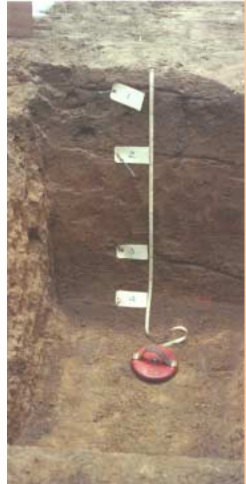
Trial pit dug through borrow area showing soil profile:
