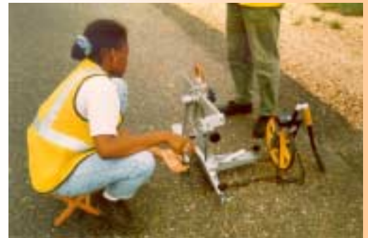
Measuring the skid resistance properties of a bituminous surface dressing.
