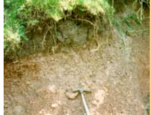
Labour based extraction is most viable when overburden soils are thin and bank deposits uncemented
