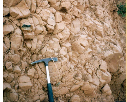
Rippable weathered hard basalt that will produce a significant proportion of hard oversize material
