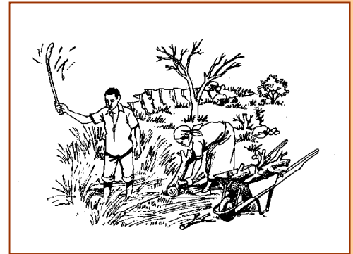
Manual methods of site clearance are encouraged, because they reduce damage to fragile tops-soil and sub-soil materials (Sketch after ILO/ASIST Bulletin No 9, 1999)
