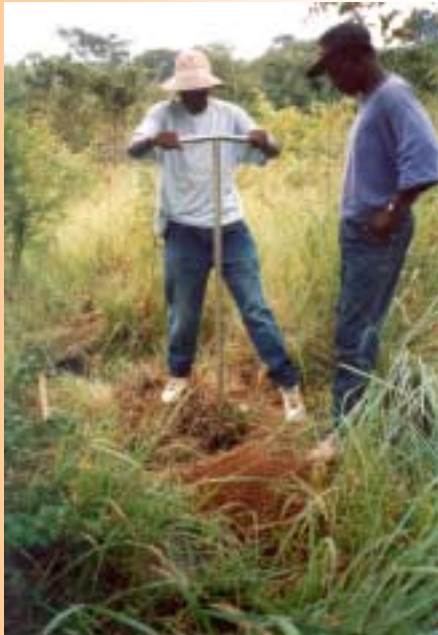
Hand auger investigation during a materials search study.
