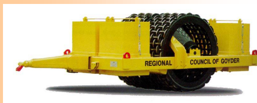
Grid roller treating oversized material on the road (Photos courtesy of Broons Hire (SA) Pty Ltd)
