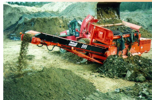
A mobile screening plant with a vibrating bar mechanism. Equipment shown is a 595 Hydratrak (Photo courtesy of Finlay Hydrascreens, Omagh Ltd.)
