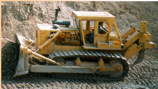
Single tine non adjustable ripper, suitable for very heavy ripping
