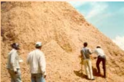
Sampling a stockpile of gravel road paving material
