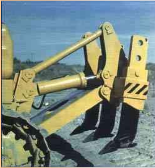
Three tine adjustable ripper
