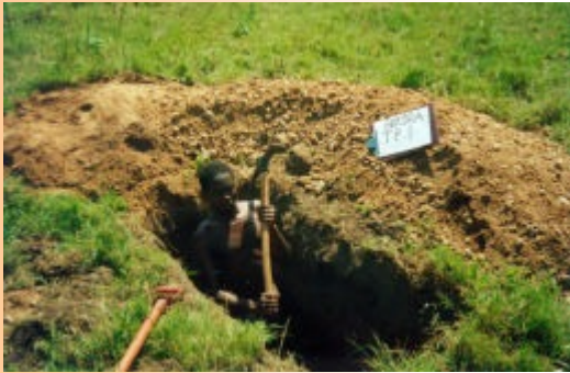
In each trial pit all layers should be accurately described and measured. Materials proposed for use should be sampled and tested.
