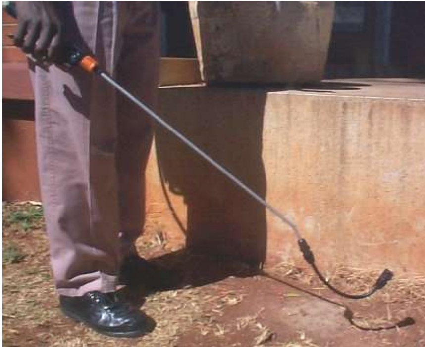
Figure 11. The Flexi lance – a flexible lance extension that can be bent in any direction and will hold its position
