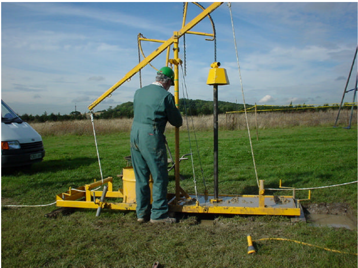
Figure 4.3 Pounder II set up and ready to drill
