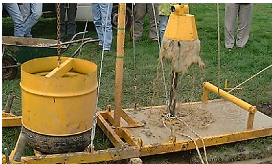
Figure 4.5 The sludging valve in action (right) and the counterbalance (left)
