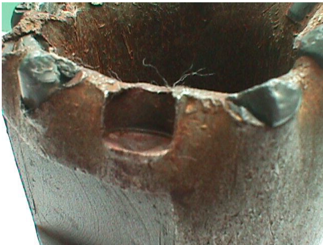
Figure 4.6 Wear to drill bit
