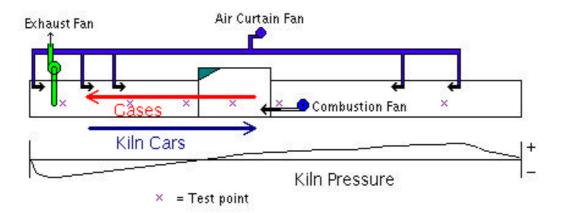
Sketch showing position of test points for measuring pressure profile in kiln:
