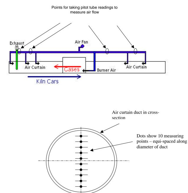
Sketch showing positions for pitot tube readings
