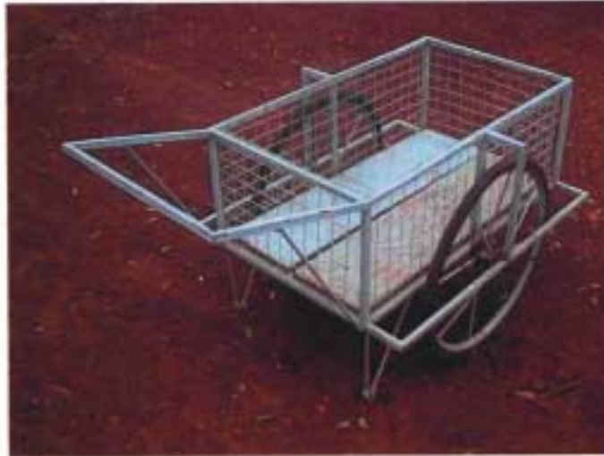
The hand cart produced by GRATIS and introduced by the IMT Project
