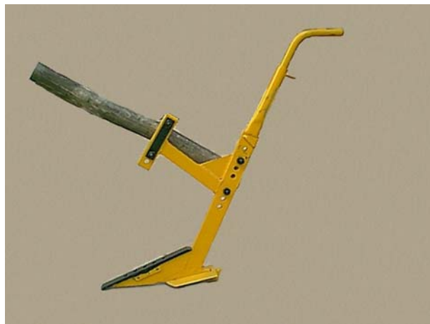
Figure 20: The winged chisel plough to improve the infiltration of rainwater
