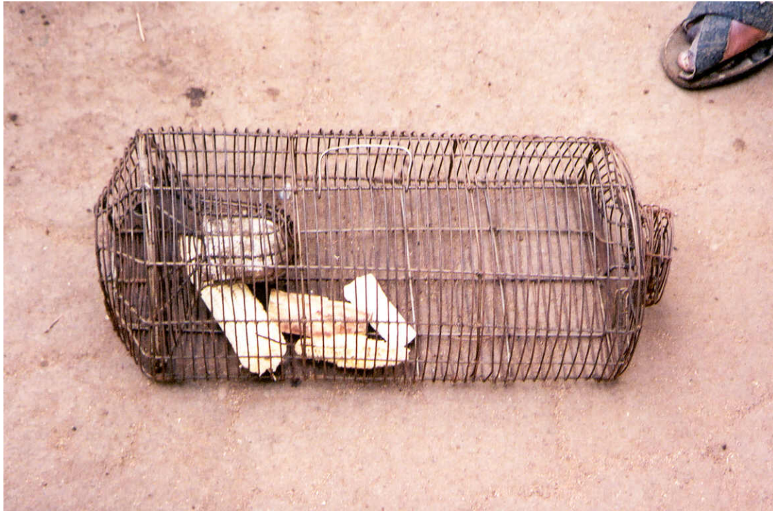
Figure 1. A Mozambican-made version of the Indian Deccan multi-catch trap. Rodents enter the trap through an opening (left side of picture), their weight triggering a treadle which allows them access to the food bait. The treadle is counter-weighted so that it closes, preventing the rodent from exiting the trap.
