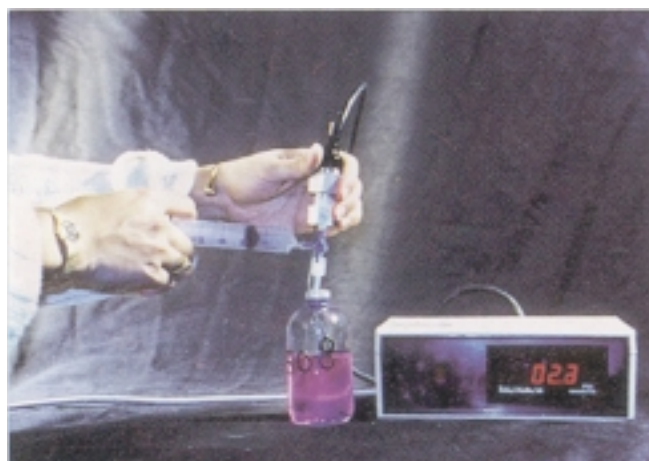
Using the pressure transducer technique for evaluating the nutritive value of tropical forages.
