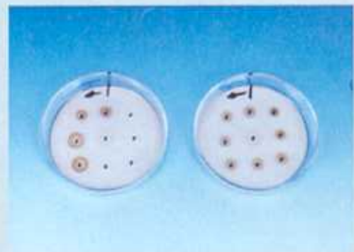
Extracted tannins assayed using the radial diffusion technique. Tannins diffuse into the agarose gel plates which contain protein. The tannins bind the protein to form dark rings which can be measured to give a quantitative measure of the activity of the tannins.
