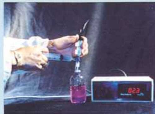
Laboratory (in vitro) gas production method. Feed samples are fermented by rumen microbes in glass bottles sealed with rubber stoppers. The mixtures are incubated at 39°C in an incubator or water bath. The picture shows the gas pressure and volume being measured using an electronic pressure meter. Gas is removed from the bottles after measurement and the bottles returned to the incubator.
