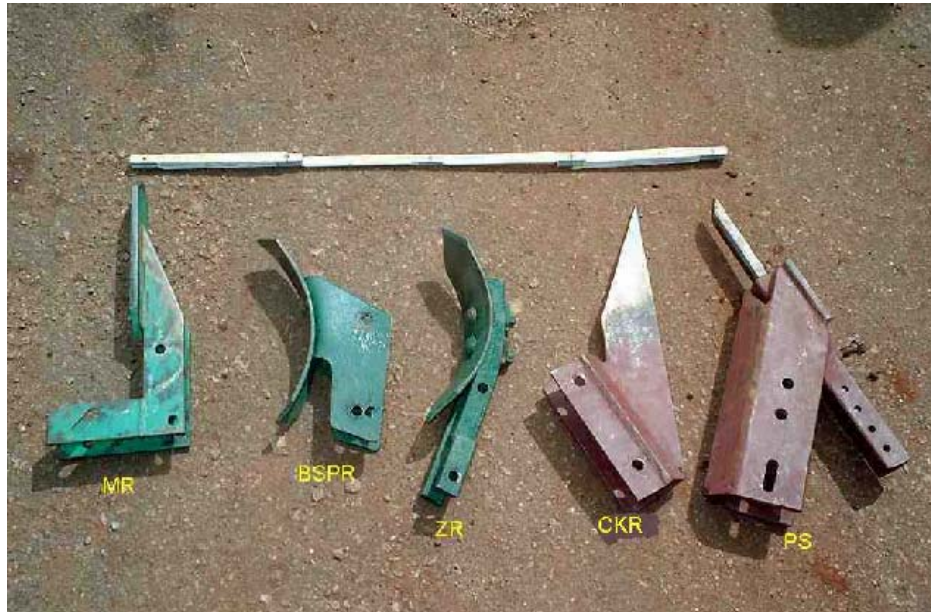
Fig 2: Designs of ripper tine evaluated
