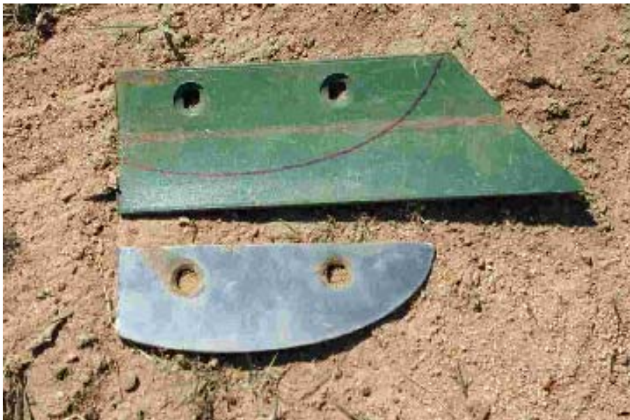
Fig 6: New and worn plough shares (profile of worn share depicted on new share)
