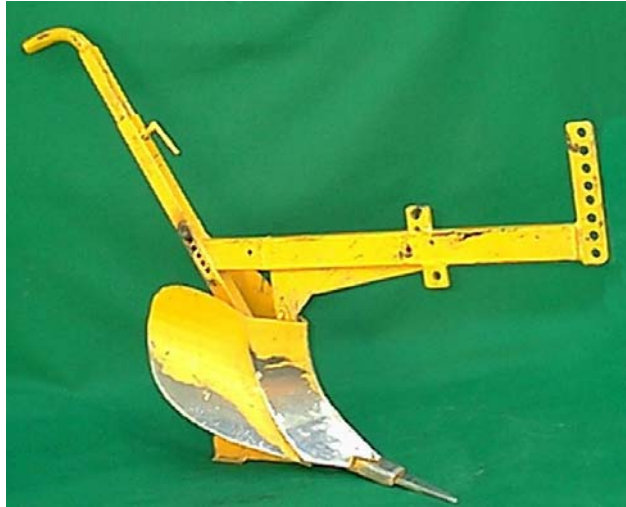
Figure 8. Scaled-down arado combinado from Bolivia, designed initially for ox-draft but now within the capability of equines.
