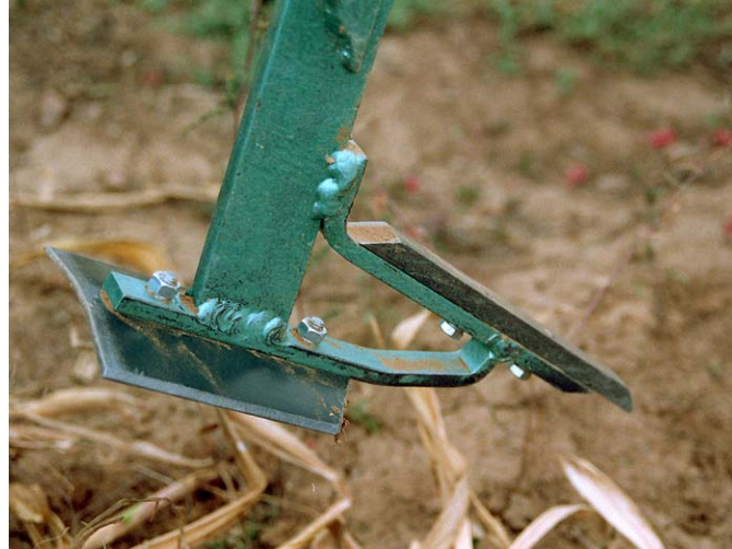
Figure 9. Wing-tined chisel plow for more efficient soil bursting during vertical tillage.
