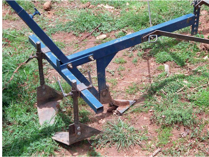
Figure 10. A three-tined cultivator designed for single-equine draft.
