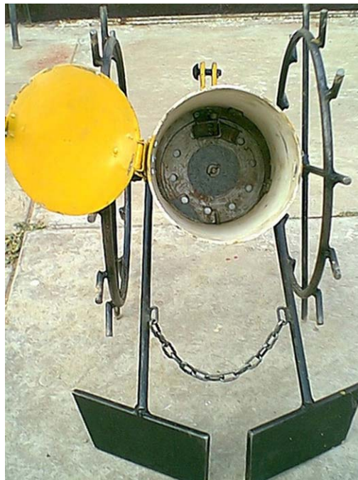
Figure 12. A horizontal plate seed metering mechanism gives more uniform seed spacing and fewer broken grains.
